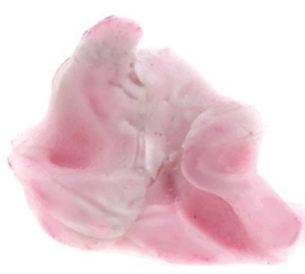
Material did not set
